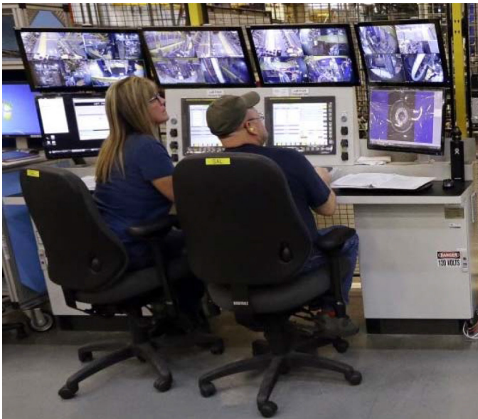
Figure 3. Remote Operator Station Controlling One Cell
